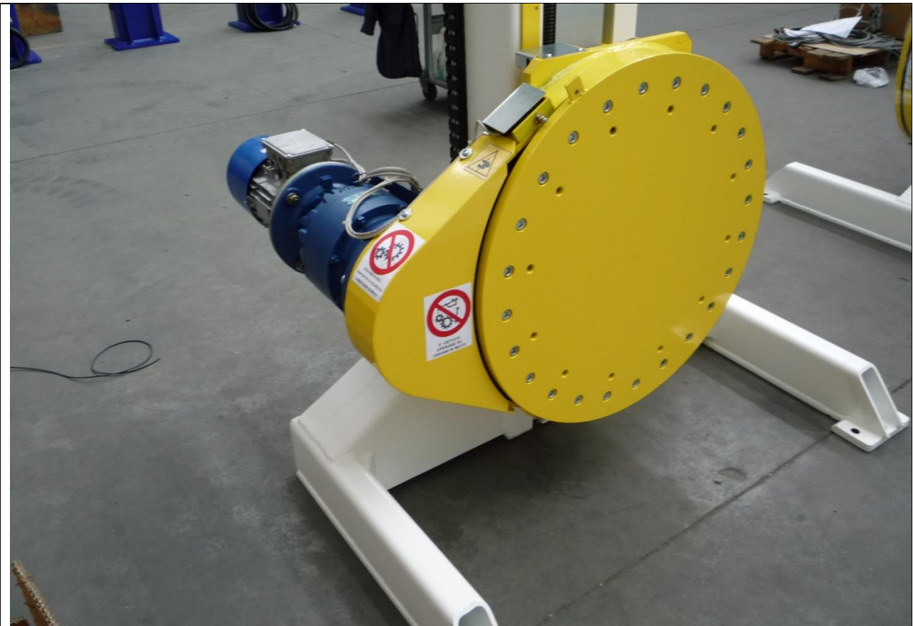
DETAIL OF MOTORIZED SLEWING BEARING ON MASTER JACK
